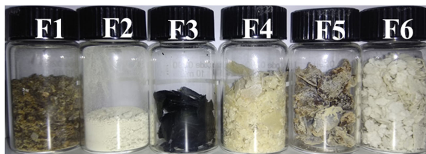
Fig. 1 Image of the end products (dry) extracted in an integrated biorefinery. F1-Salt fraction, F2-starch fraction, F3-lipid fraction, F4-ulvan fraction, F5-protein fraction, and F6-cellulose fraction
