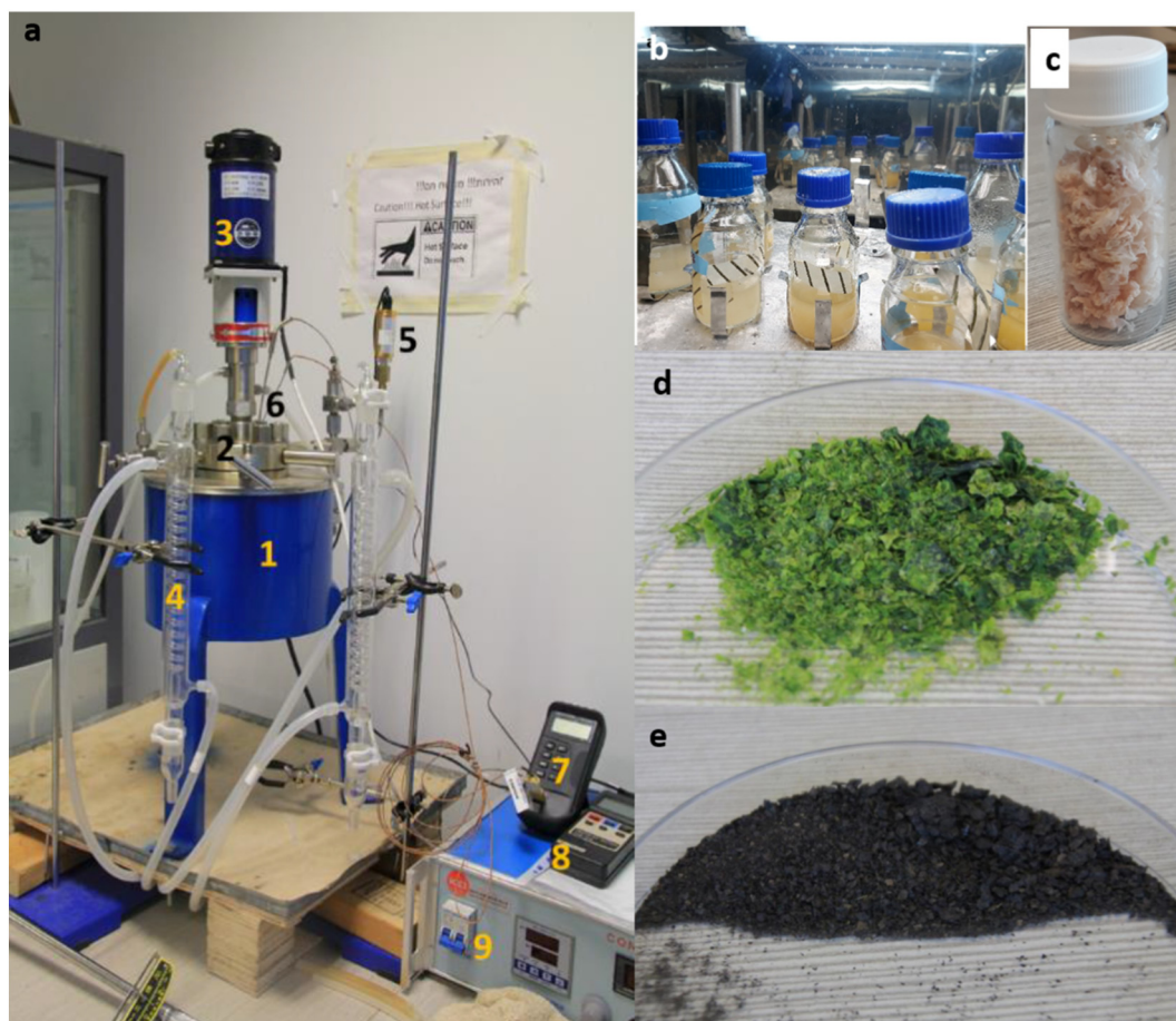
Fig. 1. (a) Dried Ulva biomass used for hydrolysis. (b) Experimental setup for PHA production using hydrolysate. (c) PHA obtained after extraction. (d) Digital image of Ulva biochar after hydrolysis. (e) Experimental setup for hydrolysis of Ulva biomass. 1. Electric heater 2. Reactor 3. Stirrer motor 4. Heat exchanger 5. Pressure sensor 6. Thermocouple 7. Temperature gauge 8. Pressure gauge 9. Controller.
