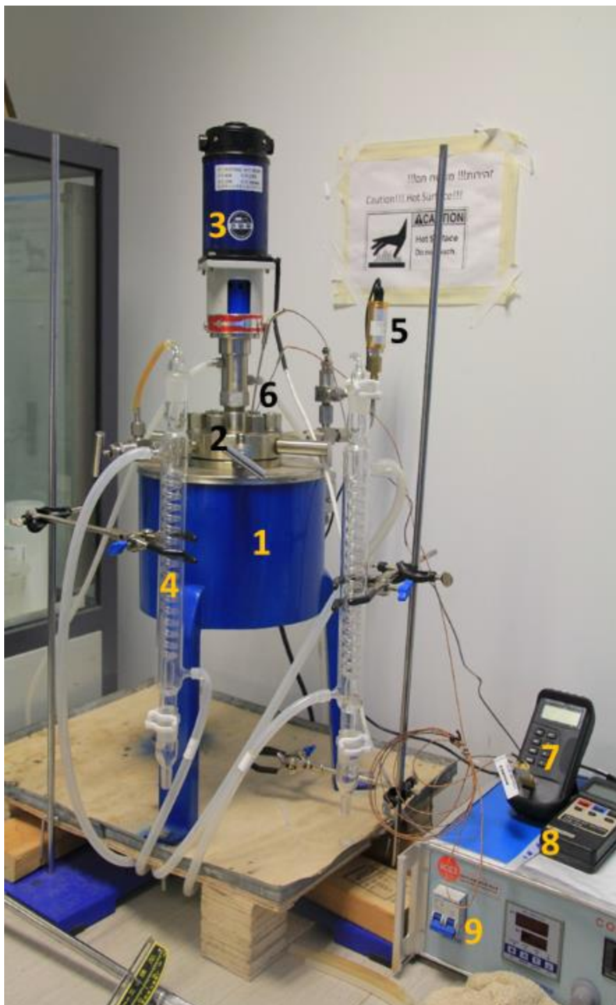
Figure 6: Actual picture of the HTL batch reactor used in this study. 1.Electric heater 2. Reactor 3. Stirrer motor 4. Heat exchanger 5. Pressure sensor 6. Thermocouple 7. Temperature gauge 8. Pressure gauge 9. Controller
