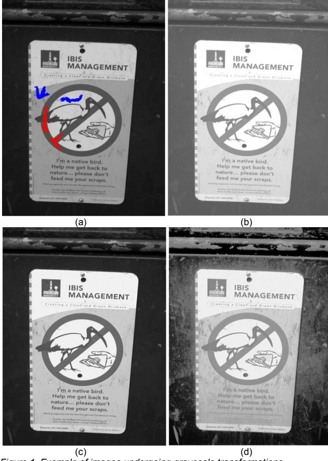
Figure 1. Example of images undergoing grayscale transformations. (a) original image with sampled foreground (in red) and background (in blue). (b) the image after brightness change (+70) (c) the image after histogram rescaling (x1.3) (d) the image after histogram equalization.
